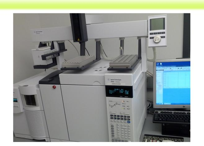
Chromatography/Mass Spectrometry with network data transfer
