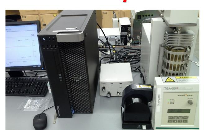
Thermogravimetric Analysis with RS-232 *instead of manual gravimetry*
